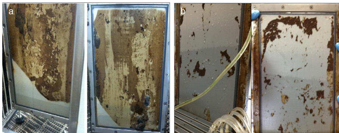
Fig. 9. FO CTA membrane fouling from long-term pilot-scale testing (a) before and (b) after introducing a parallel UF membrane operation and coarse air bubble aeration between plate-and-frame cassettes.
